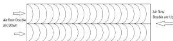
Fig. 26. Double arc rib roughness with up and down orientation
