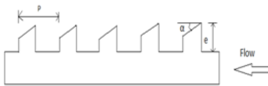
Fig. 9. Integral chamfered ribs
